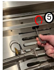
5 Use the wrench provided to change the Natural Gas orifice (1.4) by the LP Gas orifice (0.9)
