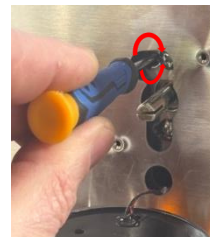
Use a flat head screw driver to adjust the height of the flame: turn clockwise = decrease height turn counter clockwise = increase height
