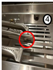
4 Place the burner on the side to access to the gas valve orifice
