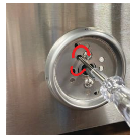
Use a flat slotted screw driver to adjust the height of the flame: turn clockwise = decrease height turn counterclockwise = increase height
