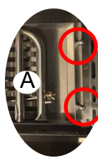
A Seat the plate on the standoffs located on each side of the Body.
